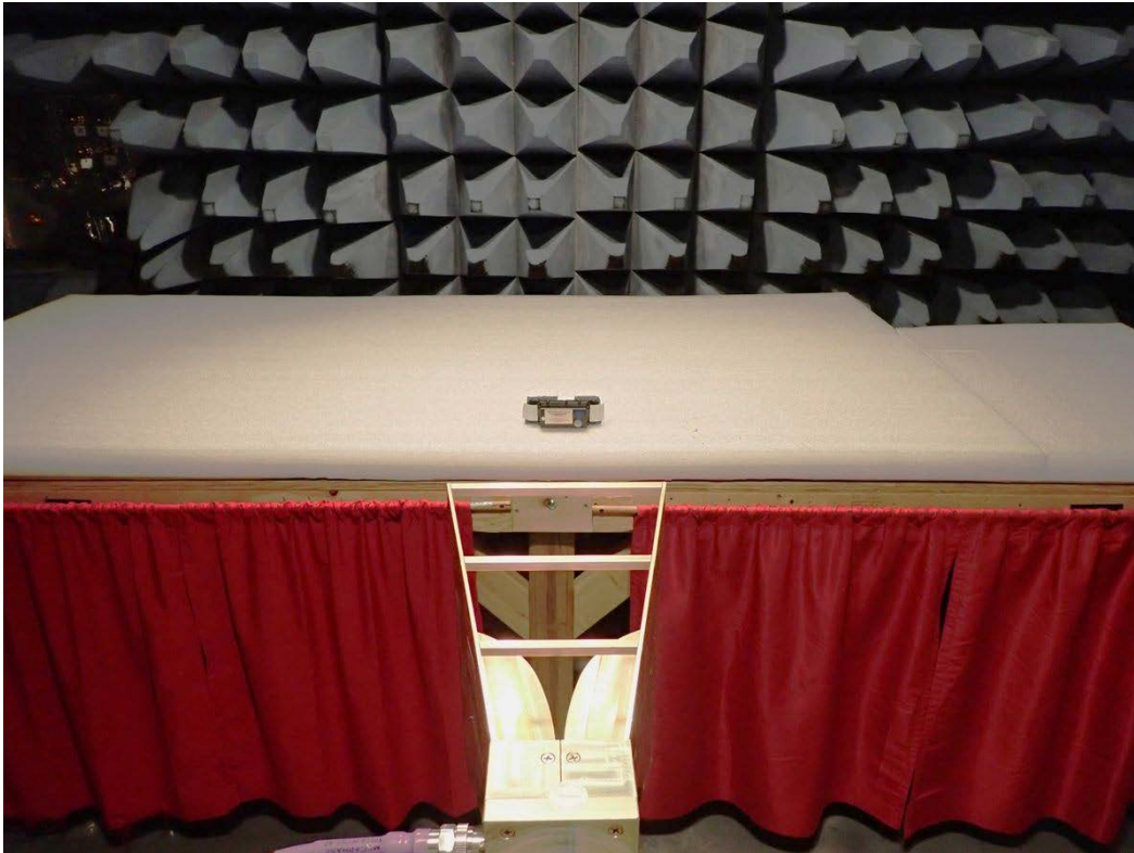
DO-160G Section 21 RE Small DRG Antenna Setup, 1GHz-6GHz, Horizontal
