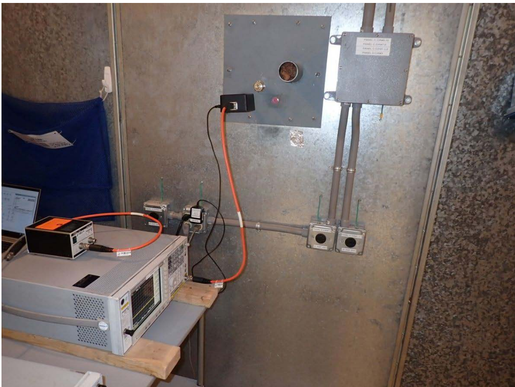
Section 21 RE Measurement Test Equipment (1 GHz - 6 GHz)
